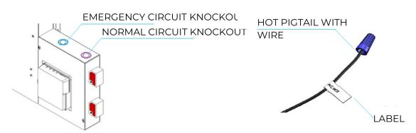
Install 3-conductor (hot, neutral, ground) 120/277 vac line for the normal circuit to the top left knockout. For the emergency circuit(s), use top-right knockout. Pigtail labeled wires with corresponding wires from input cable(s) using provided wire nut. See the table below for the label descriptions.
